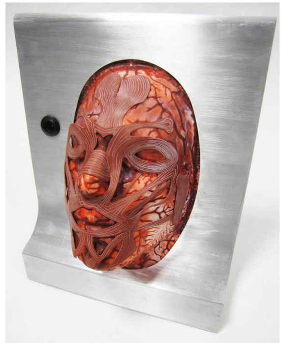
Figure 3 Animatronic model with silicone musculature
