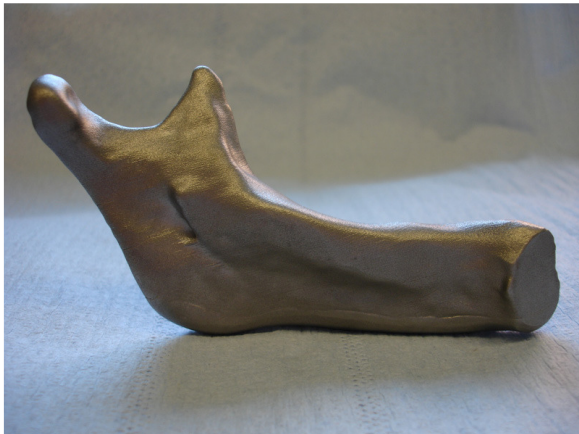
Figure 8: Physical model produced by laser sintering based on CT data.
