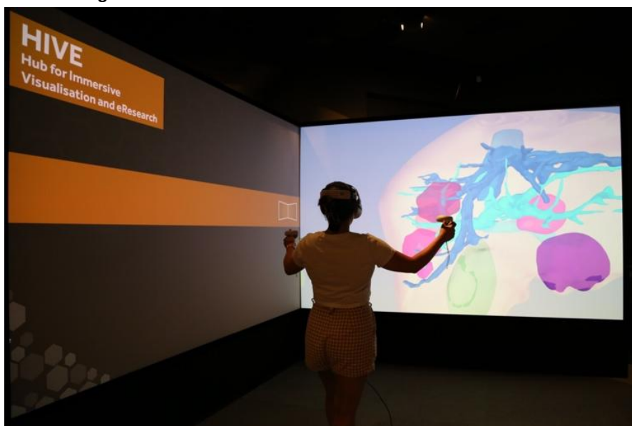
Figure 8: Virtual reality demonstration of the 3D models for the multifocal hepatocellular carcinoma case using the SlicerVirtualReality extension for 3D Slicer and the Meta Quest 2 headset and controllers. The VR view from SteamVR was displayed on the Wedge screen at Curtin Hub for Immersive Visualisation and eResearch (HIVE) for the demonstration.
