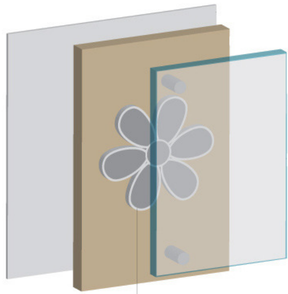
Construction of internal artwork - the images were printed using in-glass technology and positioned to allow the pattern to continue behind.
